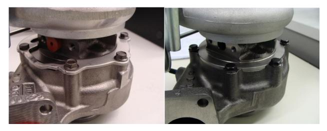
As pointed out, there are a lot of differences between an OE quality MHI turbo and a counterfeit. Counterfeiters don't have the technology, know how or resources to develop and produce a technical product as the turbocharger. When someone buy's the cheap counterfeit it will almost imminently result in damage or engine failure. The cheap solution will result in very costly problems material wise and in customer relations.
